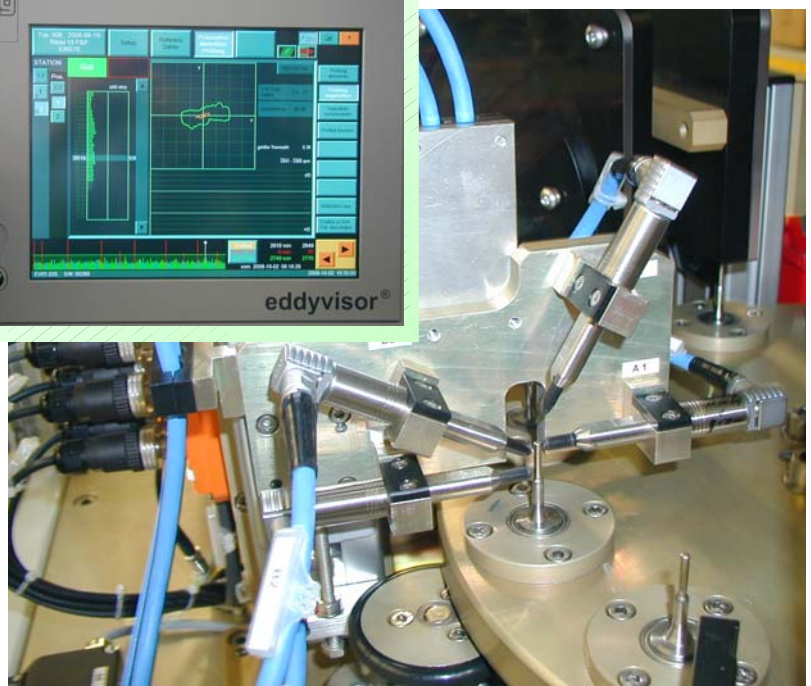
Photo: eddyvisor ® C - 4 crack detection probes at test
