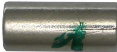
crack, partly through wall
