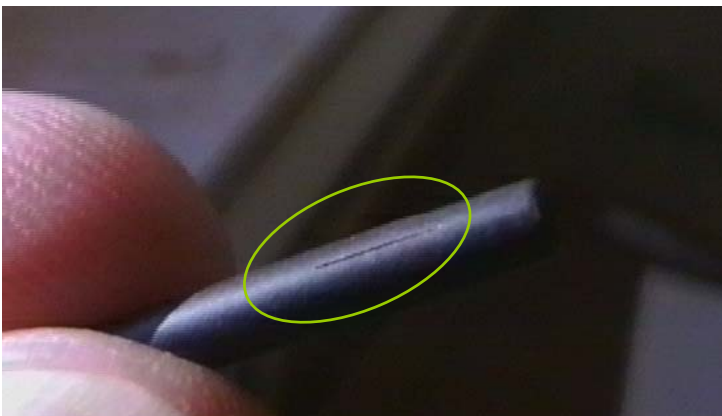
Photo 1: Test part with longitudinal crack
